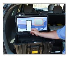
After loading feedstuffs and programming the AgriNIR to measure the defined feedstuff versus calibrated values, the unit provides a printout of results.
