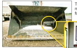
This payloader bucket at Gar-Lin Dairy Farms in Minnesota is mounted with an NIR analyzer to measure dry matter content of forages and grain, as well as protein, starch, ADF, NDF, crude fat and ash values.
