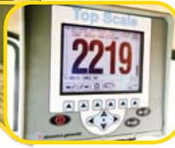
Readings from the NIR analyzer are automatically calculated with the ration balancing software and adjustments are sent wirelessly to this weighing controller for the precise amount of feed that needs to be added to the mixer. Photos courtesy of OPEN ROADS.
