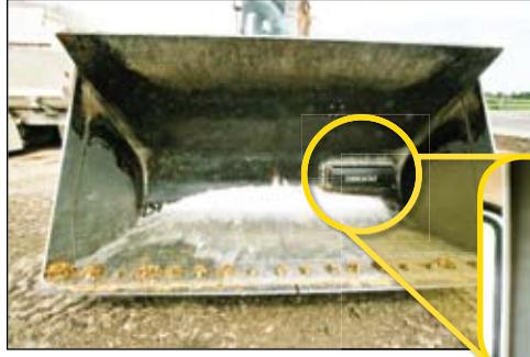
This payloader bucket at Gar-Lin Dairy Farms in Minnesota is mounted with an NIR analyzer to measure dry matter content of forages and grain, as well as protein, starch, ADF, NDF, crude fat and ash values.
