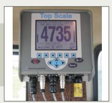
**NIR ANALYSIS:** The dg precisionFEED-ING System's NIR Analyzer, which is installed inside the bucket of a frontend loader, performs a near-infrared analysis in real time to obtain the actual composition of each ingredient in fewer than 30 seconds.
