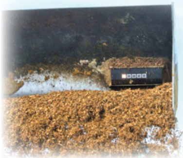
▲ Same technology installed in loader bucket to automatically suggest recipe adjustments based on results.
