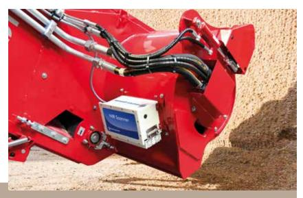
NIR analyzer for self-propelled feed mixed
